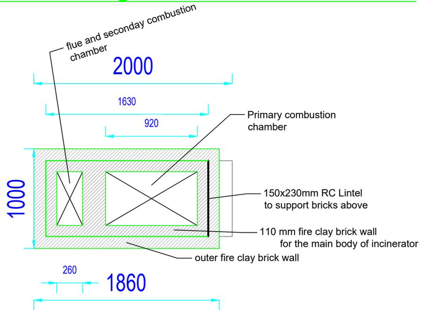
Incinerator floor plan at level 3
