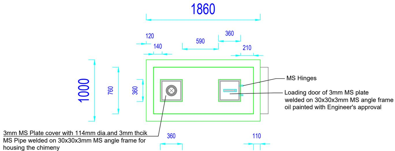
Incinerator floor plan at level 4
